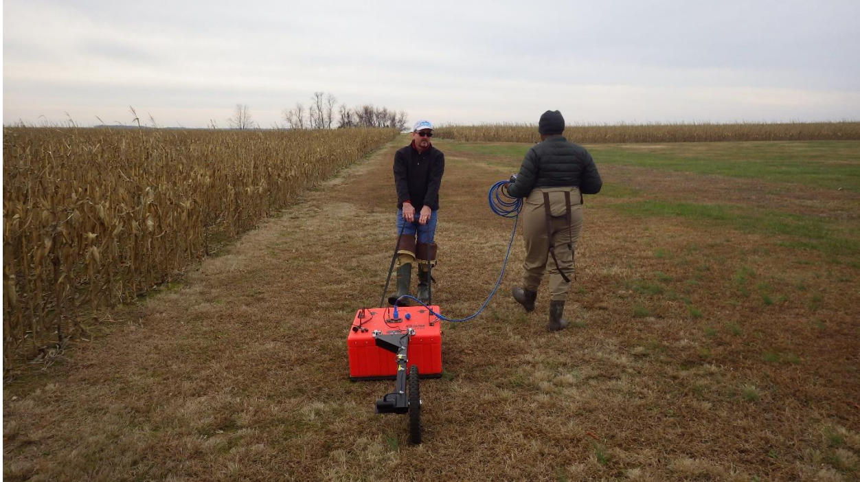
Figure 4.4. The photograph shows the ground penetrating radar sled being deployed in the interior of Parsons Island on 12-21-2019.
