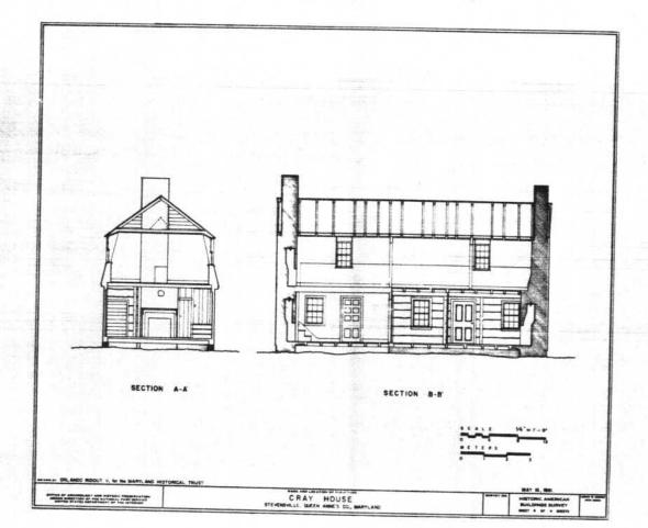
steeply pitched gable roof was replacwith the present gambrel roof. The tline of an early frame kitchen, now demolished, can be seen in the north gable of the main house.
